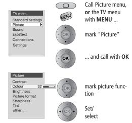
Picture settings: contrast, colour, brightness, picture format, focus, colour tone, picture adjustment, noise reduction (DNC) and automatic picture size adaptation (AMD)\*.
